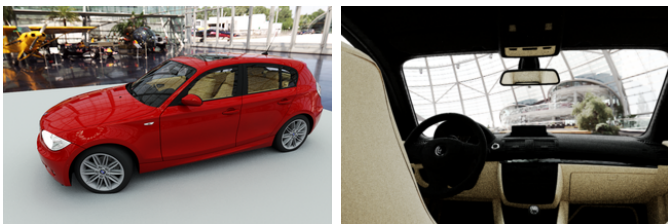
Fig. 7. A realistic path tracer operating on the car model with a variety of BRDFs (glass, car paint, Blinn, Lambertian), rendered with depth of field and HDRI environment lighting.
